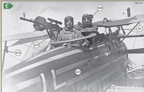
A 160hp Daimler-Mercedes D.III powered very late production Halberstadt Cl.II from Royal Prussian Schlasta 21. Note the rear view mirror, LMG 14/17 Parabellum with Oigee sight and anemometer on the port front interplane strut. The fuselage stripes are reportedly black and white but if so, they are not as dark and bright respectively as the colours used for the fuselage balkenkreuz marking. The top wing centre section appears to retain its dark brown and green stipple finish but may have been overpainted in the same colour as the dark fuselage stripes. The balkenkreuz & stripe markings on the fuselage of this and Cl.II "3" in the background are subtly different from those seen on C .
