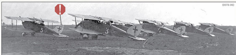
A line up of Royal Prussian Schlasta 19 Halberstadt CL.II which appear to mostly consist of late production aircraft with a mixture of post May 1918 uneven arm balkenkreuz and post June 1918 balkenkreuz. Note the overpainted cross at the top of the rudder on CL.II "5" at left and the black and white wheel markings used by Schlasta 19 at this time.
