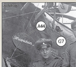
< Fuselage detail from E . Note the flat fairing (A44) over the empty generator hole and the starting magneto fairing (G7).
