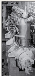
> 160hp Daimler Mercedes D.III engine. Note the thin air pump (E5) fitted at the front and external water pipe (E3).
