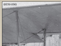
Port interplane strut detail from late production Halberstadt CLII 15342/17 seen on page 22.
