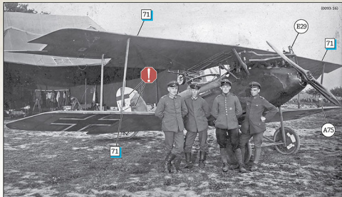
An unidentified late production 180hp Daimler-Mercedes D.IIIa powered Halberstadt Cl.II with post June 1918 converted balkenkreuz. Note the balkenkreuz painted at the top of the rudder and how the portion of the previous eisenkreuz marking on the fin was overpainted. Note the missing spinner, repair patches on the port wheel cover and under the starboard top wing tip.
