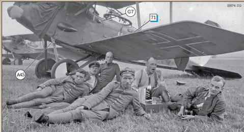
Personnel from Royal Prussian Schlasta 19 relax beside one of their very late production Halberstadt CL.II in mid to late 1918. Note "X" brace gun ring, 12.5kg PuW bomb rack under the fuselage and the overall dark appearance of the fuselage consistent with the dark green over brown stipple finish described for captured CL.II 1231/18 and subsequent Halberstadt built CL.IV. The factory applied post April 1918 balkenkreuz have been converted to the thinner, open ended, post June 1918 style.
