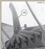
Winter cowling and exhaust detail from the unidentified mid production Aviatik built DFW C.V (Av) seen on page 29.
