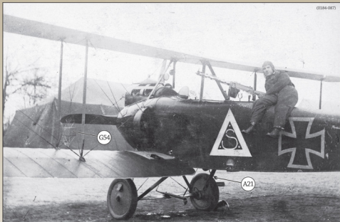
This DFW built mid production C.V from FA (A) 255 features an 'S' inside a (white?) triangle. Note the barograph (G54) + (G14b) strung between the port inner struts, extended wing walk area and that the louvered hatches of the ill fitting winter cowling have been removed. The 'ear' radiators seen here are a rarely seen 4th variation. The observer is identified in the original photograph caption as Lt Zech.
