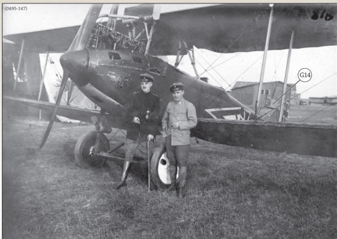
The mid production DFW built C.V 4945/16 of Seibert and Weber features several noteworthy alterations. The 'ear' radiators characteristic of mid production machines have been replaced by a central one and a captured Lewis gun has been mounted above the top wing. Note the generator attached to the starboard undercarriage strut, unusual wheel cover and the barograph (G14) strung between the port inner struts.
