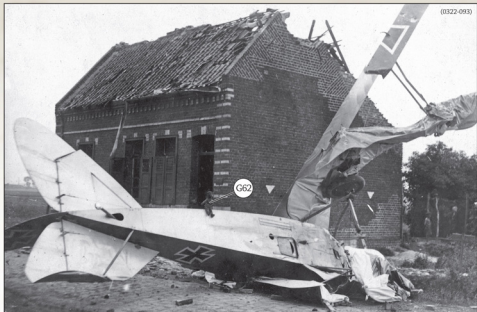
This mid(?) production DFW C.V which crashed in Brühl can be identified as LVG built by the position of the eisernkreuz centered on the control horn. A hole has been cut into the bottom of the fuselage for a camera and fitted with a jury rigged sliding hatch cover. A toy bear 662 sits on the edge of the upturned fuselage.
