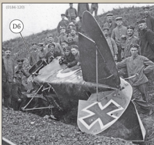
Crashed mid production LVG built DFW C.V 5232/16. Note the 'ear' radiators (D8) and LVG factory style of marking the serial number on the rudder.
