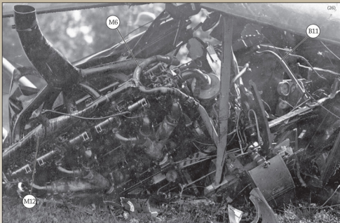
This photo of an unidentified mid production DFW C.V, probably Halberstadt built, allows us to see numerous interesting details. Note the radiator water pipes (M6), fuel & air lines on the instrument board, LMG 08/15 'Spandau' and exhaust.
