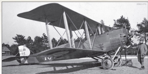
Salmson 2-A2 312 from an unidentified French Escadrille features single punch cowling louvers.
