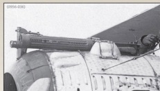
Vickers machine gun and early cowling G18 detail from A . Note the cover over the empty belt chute.
