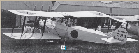
Otsu 1 295 photographed at Tachikawa. Note the polished aluminium cowling panels, black camera sight lines 10 and very dark wing struts.
