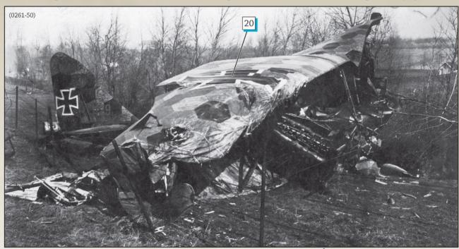
The camouflage paint has flaked off the crumpled wing exposing the bleached 'white' linen (m) fabric beneath.
