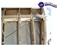
(11) Joint rib E1.And fix the wing on the installation drawing again, then pull  $\phi$  0.8mm steel wires.
