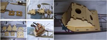
Accurately make two pairs of A2, two pcs A1 coincident with resin glue respectively. Then assemble all the parts same like the pictures.
