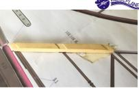
(6) Cut 6 1mm deep grooves (both ends and middle, up and down side) on the vertical fin front batten like the picture, in order to glue 1mm plywood sheet in the grooves.
