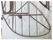
(3)Bending the 4mm stainless steel tube.
