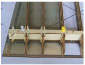
(5) Glue the ribs' strengthening plates except rib E1.
