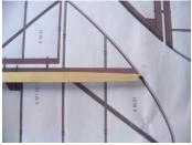
Trim the 8\*14\*300mm batten like the picture, make the diameter of the top semicircle be 4mm for connect the 4mm stainless steel tube.
