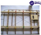
(6) Install the aileron girder, and insert&glue the strengthening plates.
