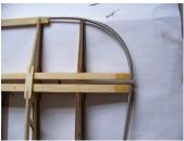
(10)Bend the 4mm stainless steel tube according to the installation drawing, then glue to the wing. Suggest using fiber cloth to strengthen the sticking-joint.
