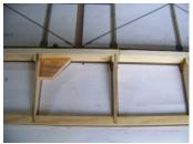
(14) Joint the strengthening plate for servo horn.
