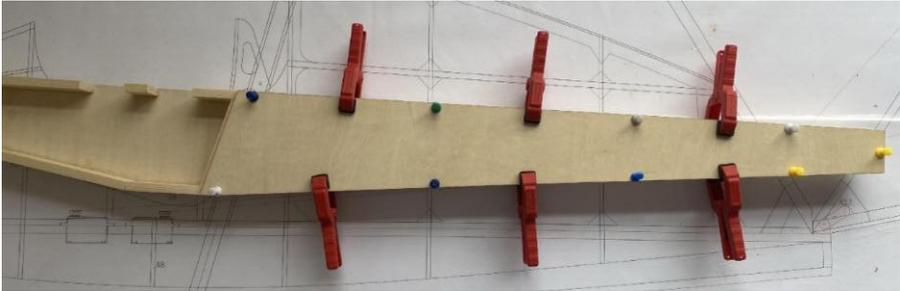
**11)Joint 12X16MM pine strips according to the drawing, and strengthen the top position with pine.**
