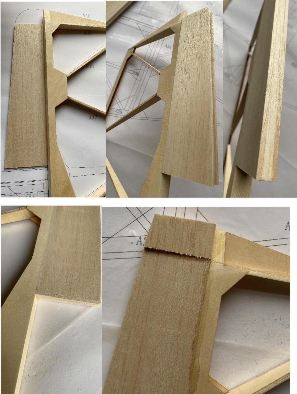
**3) The position of horns should be reinforced with pine blocks.**
