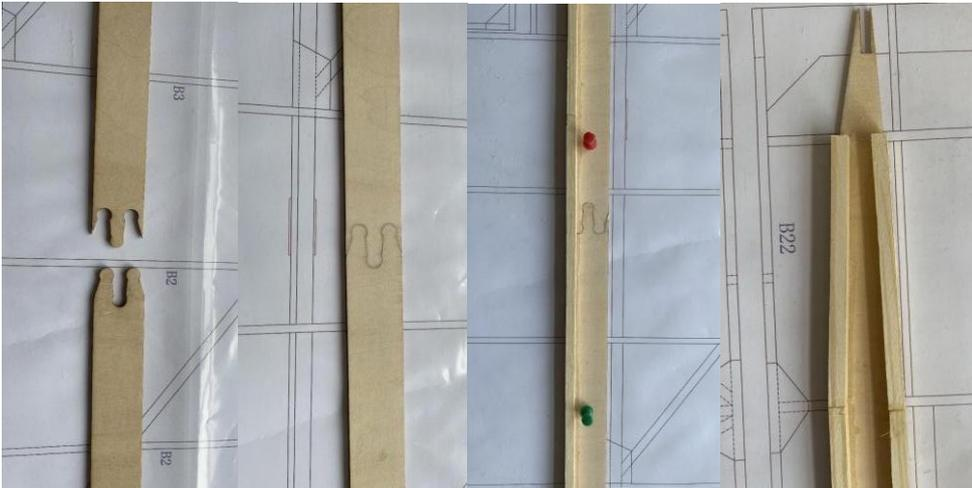
**2) Stick the reinforcing board in front and middle of girder.**
