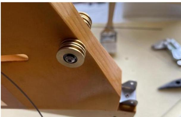
**5) Install landing skid connections with tapping screws.**
