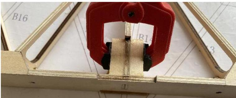
23) Stick 8MM balsa wood on the front end of the aileron and polished into triangles.
