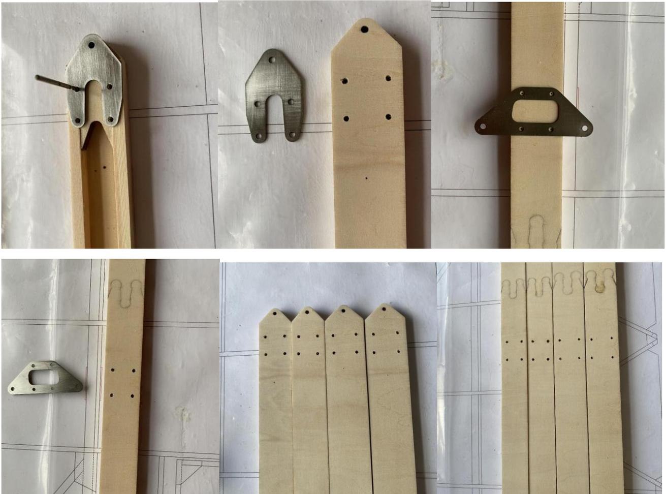
**4) Insert the ribs into the main girder according to the drawing numbers and keep the ribs vertical.**
