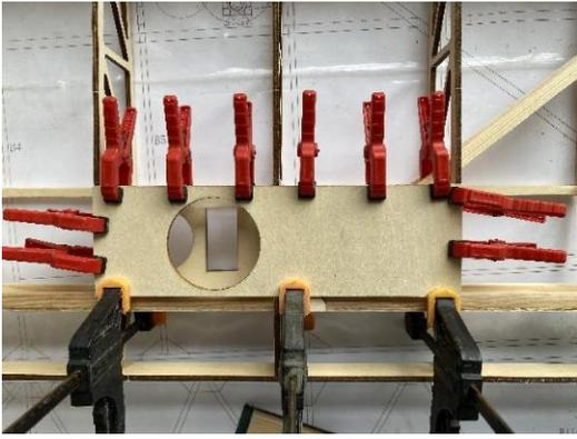
14) Stick balsa wood onto the front wing girder and smooth it.
