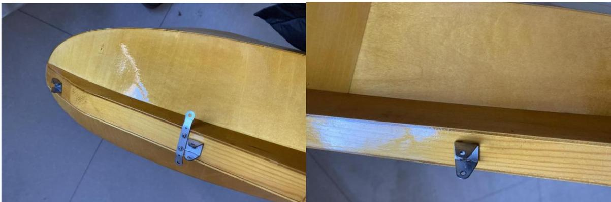
**7) Install skid to fuselage.**
