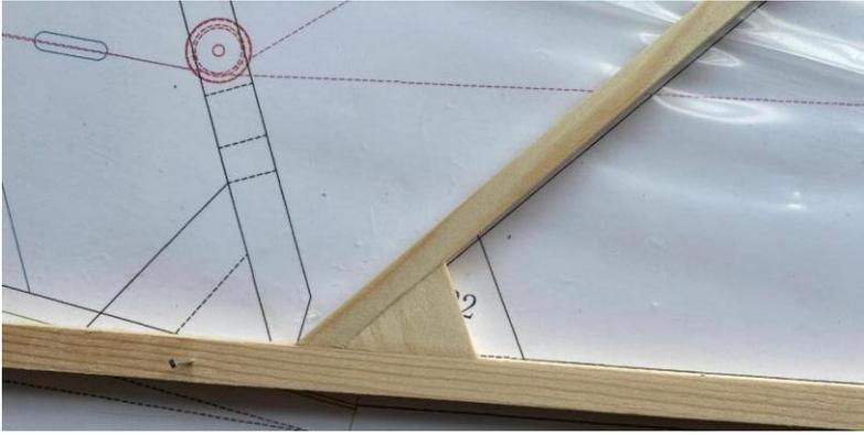
**3) Stick the reinforcement plywood with the corresponding number on both sides of the strips.**
