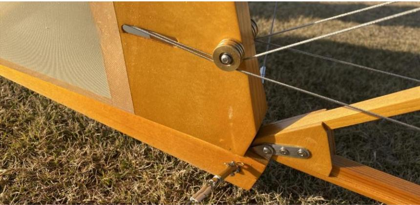
**11) Mounting for elevator pulleys.**
