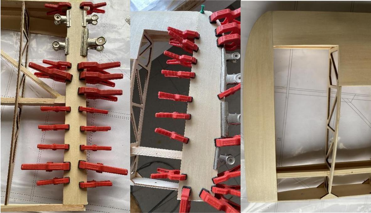
**18) Fill the joint with balsa wood.**
