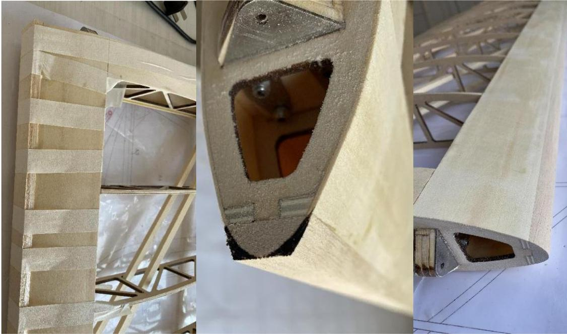
**20) Stick balsa wood at aileron connecting rod exit .**
