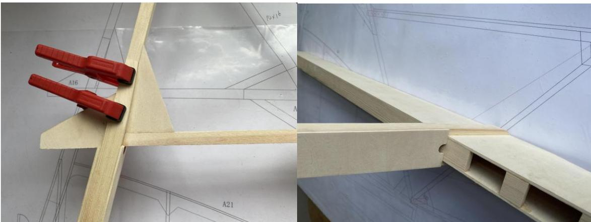
**18) Combine fuselage rear, reinforced with pine blocks.**
