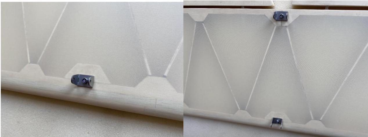
2) Assemble the tail fins on the fuselage, mark the position where need to drill a 3MM hole, keeping the perpendicularity of the holes.
