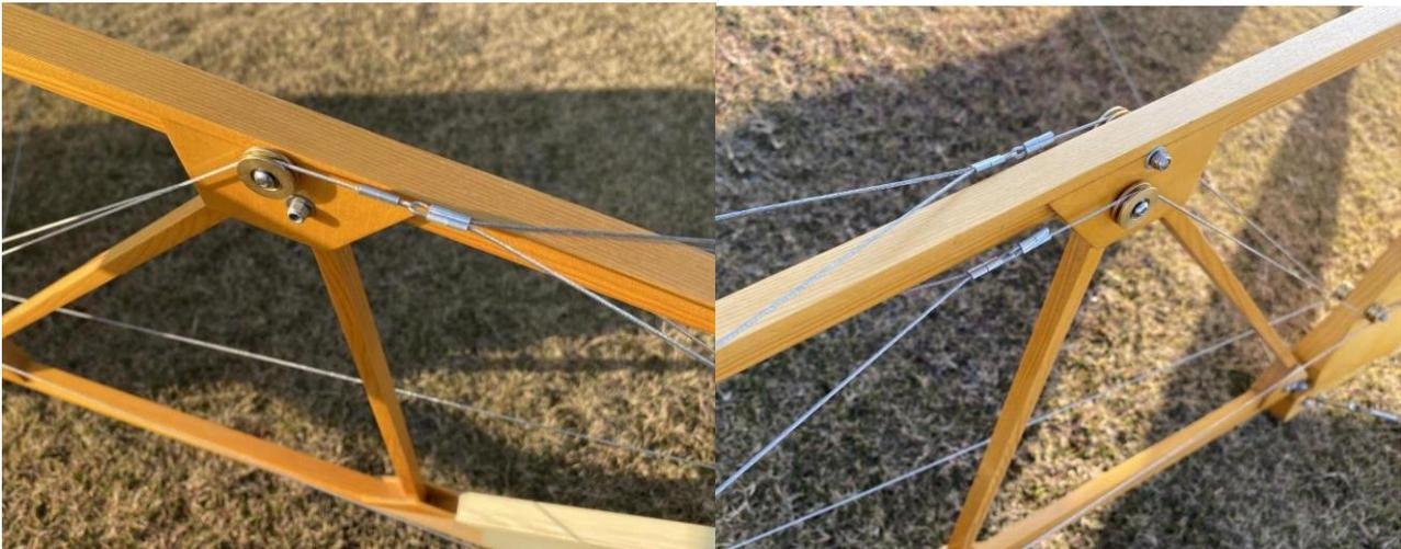
**12) Installation of the bracing wires for the fuselage and tail.**
