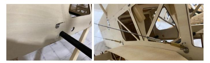
Assemble bracing wires.
