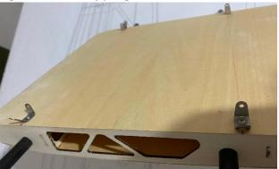
Assemble the aligning frame (for positioning the middle of the top wing) and fix it to the fuselage with self tapping screws. (The aligning frame is only temporary and will be removed in the following steps)
