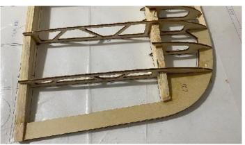
Glue balsawood on the wing ribs for additional strength when covering.
