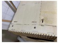
Cut off the excess of the pine strips according to the shape on the drawing. Epoxy wood parts together.
