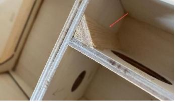
Glue the servo mounts and install the PVC tubes for the push rods.
