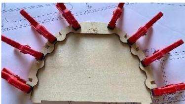
Install the formers to the fuselage.
