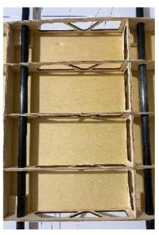
Glue 8x8mm balsa strips to the leading edge, then glue the top sheeting in place.
