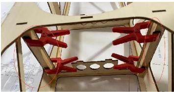
Glue 10x10mm pine strips on the fuselage bulkhead A43, A45 for reinforcement.
