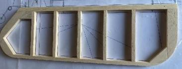
Assemble the fin over the plan.
