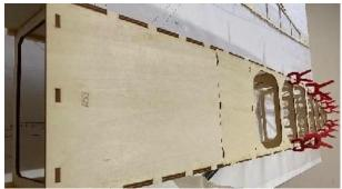
Install plywood to the upper fuselage.
