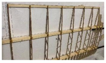
Use the template to set the dihedral angle on the first rib. Then install the PVC tubes for carbon tubes. Make sure the carbon tubes can move inside the PVC tubes freely.
