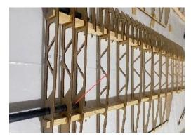
2) Glue 8x8mm balsa strips to the leading edge. Then glue the upper and lower plywood.
