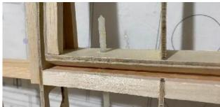
Assemble the horizontal tail over the plan.
