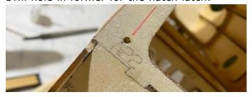
Fill the front with 8mm balsa and sand to shape
