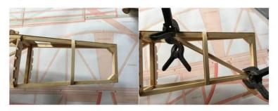
11) Stick the fuselage battens, some ones need to be butted joint and extended.
