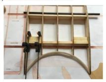
6)Paste 6X8 paulownia strips on the front spar, drill a 3MM hole in the spar according to the position of the drawing, and insert the 4-claw nuts.
