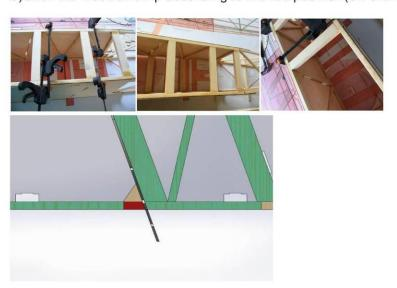
6) Stick the fuselage bar according to the drawing, and keep the frame vertical.
