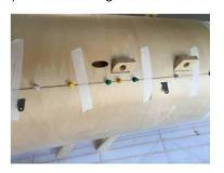
26) Use the A17 wing rib as the template, mark the fuselage cover, then cut the redundant parts and paste the balsa wood and polish.
