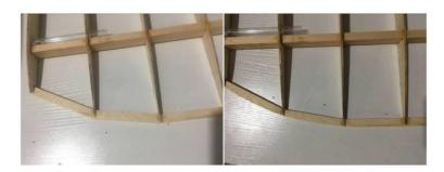
8) Fill the main girder with tung wood strips, polish and flatten it, and stick 1MM plywood.
