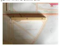
5)Install the four-claw nuts, fix with resin glue, and remove the excess with a file.
