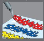
To apply the decals, place one end down, hold the other end up, and gradually smooth the decal down with your finger as you go. This will prevent air bubbles. Placing both ends of the decal down and then trying to smooth it out will result in air pockets. Look at the photos on the box for typical decal placement.
