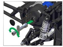
noise. From the factory, the slipper clutch adjusting spring is fully compressed for best drag racing results. Remove the rubber slipper clutch plug on the transmission cover to adjust the slipper (if needed). Use the 4-way wrench to turn the adjusting nut clockwise to tighten and counterclockwise to loosen.
