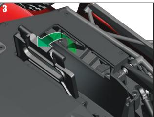
4. Insert a fully charged battery pack into the battery compartment. Place the second battery on top of the first.
