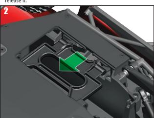
Flip the hold-down up to access the battery compartment. Rest the battery hold-down against the chassis in the open position.
