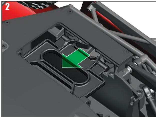
3. Flip the hold-down up to access the battery compartment. Rest the battery hold-down against the chassis in the open position.
