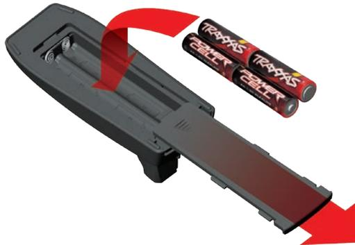
1. Remove the battery compartment door by pressing the tab and sliding the door open.
