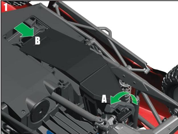
2. Pull the battery hold-down toward the center of the truck to release it.
