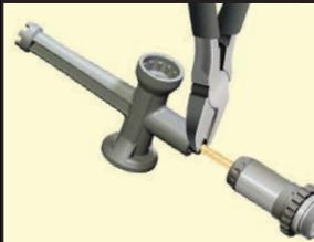
C. Remove/Install Rod End
