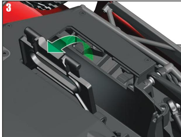
4. Insert a fully charged battery pack into the battery compartment. Place the second battery on top of the first.
