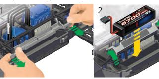
**Note:** The battery compartment will accommodate the Traxxas 6700mAh 4s battery pack (part #2890X). When using other LiPo batteries, additional foam blocks and battery pack spacers are required for proper fitment (see battery chart).
