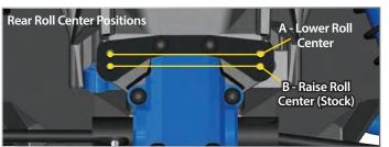
Note: If you place the front links in the bottom position (not stock), then the pivot balls in the steering will need to be flipped. The outer pivot balls come out of the box in the lower position (A). When the roll center is moved, the offset will need to be flipped (B).
