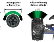
high speed, or on tracks that favor sweeping turns where gentle steering inputs are required. The ranges are exaggerated for illustrative purposes.
