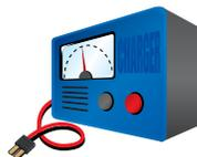
NiMH battery charger (peak detecting type recommended) *see sidebar*
