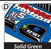
7. When the LED turns solid GREEN, programming is complete. The LED will continuously shine green indicating the XL-5 is on and at neutral (D).
