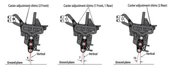
The stock caster setting is 7-degrees with one shim at each end of the arm. Reduce the caster angle to 4-degrees by removing the rear shim and inserting it next to the front shim. The caster angle can be increased to 10-degrees by removing the front shim and inserting it next to the rear shim.
