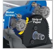
Incorrect gear mesh is the most common cause of stripped spur gears. Gear mesh should be checked and adjusted anytime a gear is replaced. Access the gears by removing the single screw on the top gear cover.
