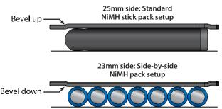
Note that one side is labeled "25" and other side is labeled "23". The 25mm side is for use with typical stick type battery packs. If you are using side-by-side racing packs, simply flip the hold-down over to the 23mm side and use it on the opposite side of the chassis. Accessory hold downs and foam (part #3927X) are available to accommodate larger battery packs. See the 3903 E-Maxx parts list for more information.
