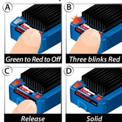
4. The LED will blink and then turn solid green (Low-Voltage Detection ACTIVE) or red (Low-Voltage Detection DISABLED). The model is ready to drive.
