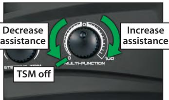
**Note:** TSM is deactivated automatically when driving or braking in reverse.
