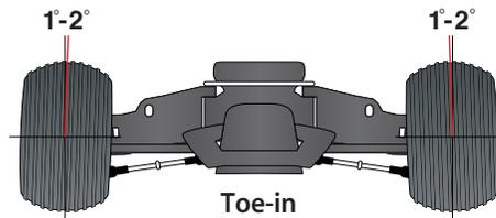
For increased stability add one- to two-degrees of toe in to each front wheel. Use the turnbuckles to adjust the alignment.
