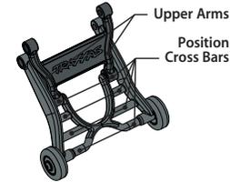
Pos. #1: The highest angle of the wheels (lowest position on the cross bars). Allows the vehicle to tip back the most for longer wheelies.
