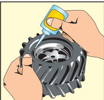
**2.** Use your thumb to push the side of the tire away from the rim. Place one or two drops of CA glue into the opening and release the tire. Capillary action will draw the glue around the bead of the tire.
