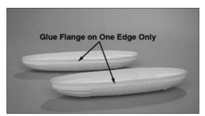
2. Trim off the excess plastic to the cut lines on the inside of the tank with scissors or a hobby knife. Use 220-grit sandpaper to even up the edges of the glue flange.
