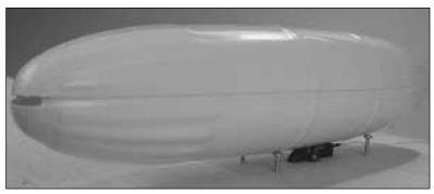
☐ 4. Install the tank on the Release Mechanism and tighten or loosen the #4 x 5/8" screws until you get the desired tank position. Ideally, the tank should have a slightly negative attitude so that it falls away from the airplane as soon as it is released. Wick thin CA on the screws to keep them from moving.
