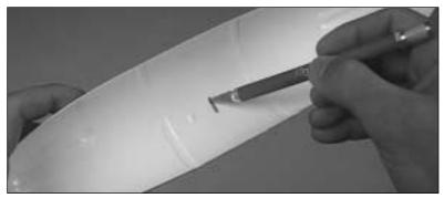
5. Cut out the slot in the top half of the tank to allow the **Release Loop** to exit through the top of the tank from the inside.
