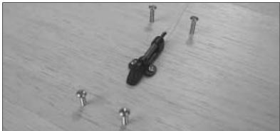
☐ 3. Drill two 1/16" holes for the Release Mechanism's mounting screws. Using the sketch above as a sample, drill four holes for the drop tank positioning screws. The location of these screws will vary from airplane to airplane. Use thin CA to harden all the holes. Install the mechanism with two #2 x 3/8" screws included. Install the four #4 x 5/8" sheet metal screws included at the outer holes. These screws will be used to position the tank in the correct attitude.
