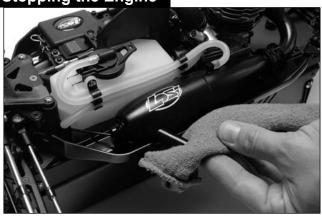
To stop the engine, use the handle of a screwdriver or a rag to cover the exhaust pipe exit (fig.), being EXTREMELY careful not to burn your hand as this will be hot.
