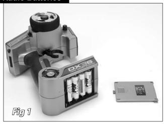
Install the 4 AA-size alkaline batteries (included) in the transmitter making sure the positive (+) and (-) negative ends are oriented correctly.
