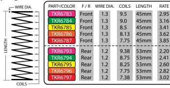
Softer springs will increase traction through the turns by allowing more roll, slow down the responsiveness of the vehicle, and can be better in the bumps. Stiffer springs will increase corner speed if traction is available and will also tend to jump and land better. Once you find a set of springs you like you will typically only change them for tracks with dramatically different conditions.
