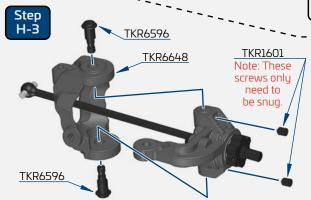
Note: Pre-thread the kingpin screws into the spindles prior to installing them into the spindle carriers. This will ensure there will be no binding.
