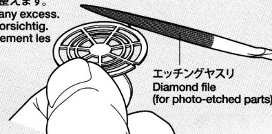
エッチングヤスリ Diamond file (for photo-etched parts)
