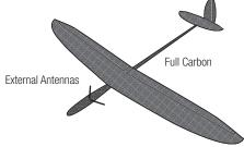
Slide the feeder antennas through the holes until the 31mm tip, and about 2mm of coaxial, completely exit the fuselage. Use a drop of CA or tape to fix the antenna to the fuselage.
