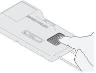
can come in handy if the receiver needs to be mounted in a location that is difficult to access, in which case a servo extension may be used for binding. If using a bind plug, remove after binding to prevent the system from entering bind mode the next time the power is turned on.
