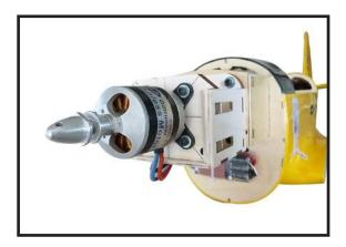
5) Attach the speed control to the side of the motor box using two-sided tape and tie wraps. Connect the appropriate leads from the speed control to the motor. Make sure the leads will not interfere with the operation of the motor.
