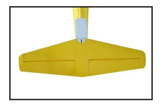
$\Box$  4) With the stabilizer held firmly in place, use a pen and draw lines onto the stabilizer where it and the fuselage sides meet. Do this on both the right and left sides and top and bottom of the stabilizer.
