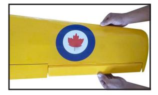
5) Turn the wing panel over and deflect the aileron in the opposite direction from the opposite side. Apply thin C/A glue to each hinge, making sure that the C/A penetrates into both the aileron and wing panel.
