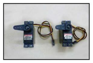
**Minimum servo spec. Torque** : 80 oz-in (5.8 kg-cm) @ 4.8V; 100 oz-in (7.2 kg-cm) @ 6.0V
