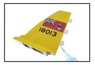
1) While holding the vertical stabilizer firmly in place, use a pen and draw a line on each side of the vertical stabilizer where it meets the top of the fuselage.
