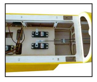
RUDDER PUSHROD HORN INSTALLATION.
