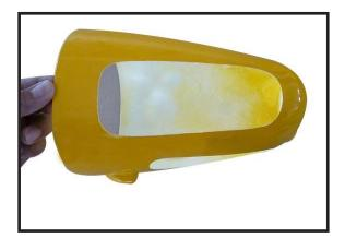
1) Tape the cowl to the fuselage using low-tack tape.
