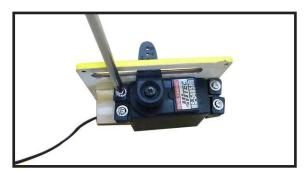
6) Apply 1-2 drops of thin C/A to each of the mounting tabs. Allow the C/A to cure without using accelerator.
