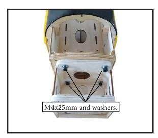
4) Attach the motor mount to the front of theelectric motor boxusing four 4 mmblind nut, four M4x20 mm hex head bolts to secure the motor. Please see picture shown.
