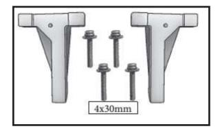
2) Use four 4x30mm head bolts and four 4mm washers to attach the engine mount rails to the fiewall. Tighten the screws . Make sure to use threadlock on the screws to help prevent them from vibrating loose.
