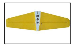
$\Box$  7) When you are sure that everything is aligned correctly, mix up a generous amount of 30 Minute Epoxy. Apply a thin layer to the top and bottom of the stabilizer mounting area and to the stabilizer mounting platform sides in the fuselage. Slide the stabilizer in place and realign. Double check all of your measurements once more before the epoxy cures. Hold the stabilizer in place with T-pins or masking tape and remove any excess epoxy using a paper towel and rubbing alcohol.
