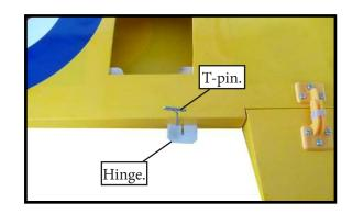
3) Slide the wing panel on the aileron until there is only a slight gap. The hinge is now centered on the wing panel and aileron. Remove the T-pins and snug the aileron against the wing panel. A gap of 1/64" or less should be maintained between the wing panel and aileron.
