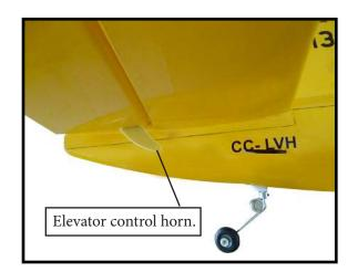
3) Thread one clevis and M2 lock nut on to each elevator control rod. Thread the horns on until they are flush with the ends of the control rods.
