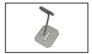
2) Remove each hinge from the wing panel and aileron and place a T-pin in the center of each hinge. Slide each hinge into the wing panel until the T-pin is snug against the wing panel. This will help ensure an equal amount of hinge is on either side of the hinge line when the aileron is mounted to the aileron.
