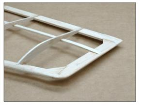
Open slots in R0 with a 1/8 in. drill to form hole for wing mount bolt.
