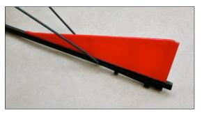
Using a 0.025 drill, open hole for rudder hinge in center of notch at end of boom.
