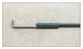
Install pushrod with Du-Bro RC Micro E/Z Links [DUB849]. Center servo, and adjust pushrod length by sliding metal fitting in/out of heat-shrink sleeve.
