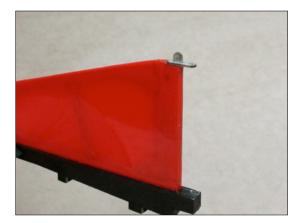
Using 0.025 wire, make a 90 degree bend 1/8 in. from one end. Trim wire to 2-3/8 in. to form rudder hinge pin.
