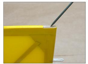
☐ Fit control horn R6 to rudder. Note that short arm of horn is marked "R" and extends on the right side of rudder. *Ensure that control horn is square and perpendicular to rudder.* Tack with thin CA.
