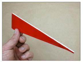
Remove covering from hinge mount area at base of stabilizer. Do not install hinge at this time.
