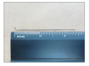
Insert hinge pin through rudder hinge tabs trapping boom. Pass wire through hinge tabs at bottom of rudder and vertical stabilizer.
