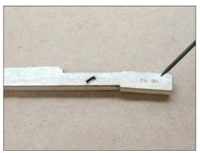
Using guide slots in F1b, drill 1/8 in. hole for wing mount.
