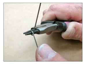
Ends of wire should diverge about 45 degrees. Refer to plan for proper angle. Trim straight portions to 1 in. length.
