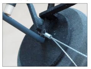
Close close crimp with round nose jewelers pliers. Squeeze crimp in two places, and secure with a small drop of medium CA. Trim off excess wire.
