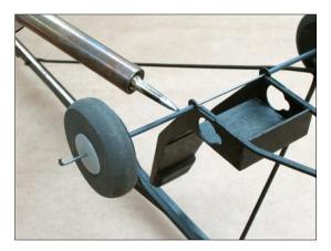
Fit nose wheel strut to F1 and seat struts. Tack with thin CA glue.
