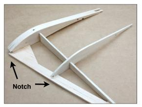
Fit trailing edge W2 to ribs R1 and R2.
