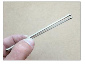
Seal strut and paint black at this time. Leave tabs unpainted, to provide a good wood to wood bond with the fuselage boom.
