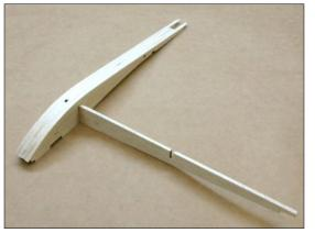
With rib/spar assembly flat on the table, fit leading edge W1 to R1 and spar S1. Tack glue with medium CA.
