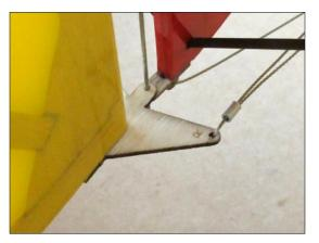
Attach second wire to <u>left</u> side of control horn. Snug wire but do not crimp.
