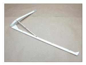
Fit rib R2 to leading edge and spar. Note All ribs are stepped at the leading edge producing a 1/8 in. notch above W1that will receive the W4 leading edge doubler.
