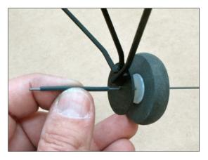
Next, slide seat onto axle. *Ensure seat is facing forward!*
