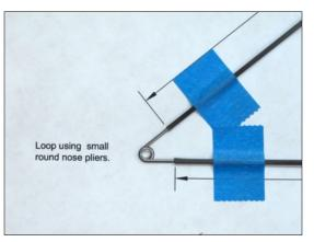
□ □ Insert long end of bent wires into tubes. Carefully check finished length of struts. Adjust tubes and wires as necessary. Tack glue with thin CA.
