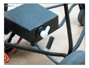
Cut a length of 1/16 in. dia. carbon rod 11 in. long to make elevator pushrod.
