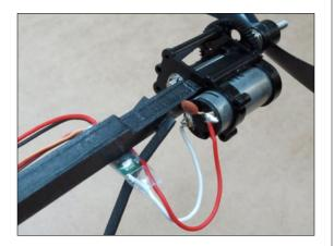
**Note:** We recommend removing the connectors from the motor and speed control, reducing the length of wire, and directly soldering both components together.
