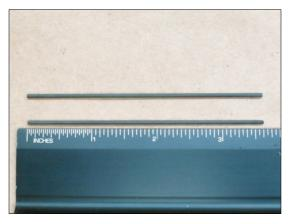
☐ Fit struts in holes in stabilizers. Trim to fit if necessary. *Ensure vertical and horizontal stabilizers remain perpendicular to each other.* Bond with medium CA.
