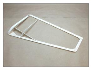
Fit and bond ribs R3, R4 and R5 to wing assembly.
