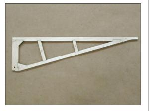
Lightly sand vertical sub-fin, rounding lower edge. Leave upper edge and trailing edge square.
