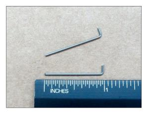
Join fittings to pushrod with a 1/2 in. length of 1/16 in. heat-shrink tube. Shrink tube using a fine tip soldering iron. DO NOT GLUE.
