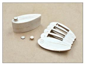
Sand tank smooth, round edges, seal with Deft and paint white.
