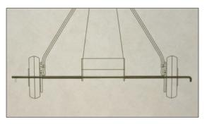
Cut two lengths of 1/16 in. heat shrink tubing 1-3/8 in. long to make axle spacers.
