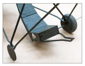
Now, slide remaining spacer onto axle and extend axle through the right hub.
