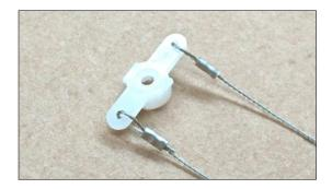
Electronically center rudder servo and mount horn as shown.
