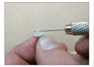
Open holes for fittings in wing using a fine point soldering iron.
