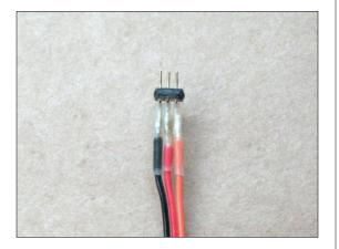
Remove connector from speed control. Trim wires for a finished length of 11 in. and solder on extension. *Ensure colored wires match.*
