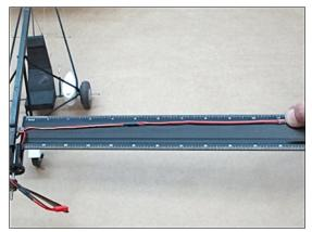
Route lead down the left forward strut. This simulates the fuel line routing on the full size aircraft. Retain with hot glue.
