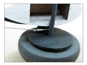
Rig seat to fuselage boom in the same manner. Pass wire over boom and pinch with fingers to shape close to boom. Again, do not pull rigging too tight, as this may break the seat.
