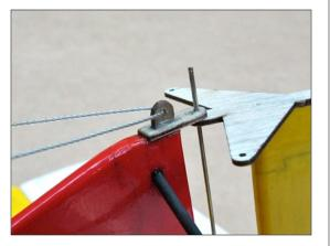
☐ Slide on another crimp, and secure wire to other end of strut as before. **Note:** Do not pull tail rigging too tight, as this will pull the tail surfaces out of alignment.
