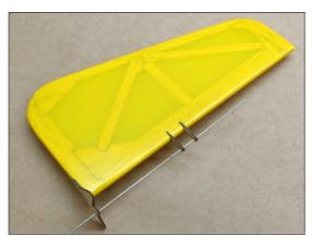
Carefully align wire/hinge line with centerline of rudder, and parallel with rudder leading edge. Bond hinges and control horn to rudder with medium CA. Remove wire.
