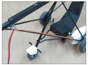
Plug lead into receiver. Ensure connector is oriented so black/ground wire is plugged into black/ground socket on receiver.
