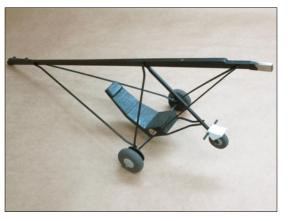
Fit vertical stabilizer to slot on bottom of fuselage boom. Ensure stabilizer is aligned with the vertical centerline of fuselage and bond with Medium CA.
