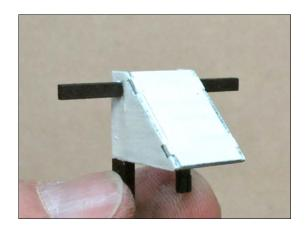
Fit fender assembly to nose wheel strut. Align carefully and bond with medium CA.
