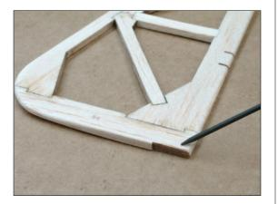
Cover rudder with AeroLITE or AeroFILM. Open slots for hinges with hobby knife or razor blade.
