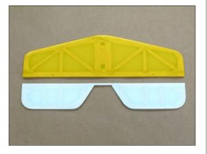
○ With low-tack masking tape, secure stabilizer and elevator to table as shown. Leave approximately 1/32 in. gap between surfaces.
