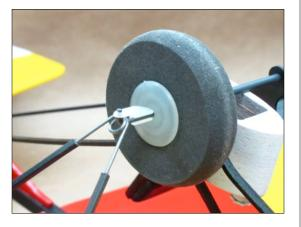
□ Insert strut into fitting and secure with a Du-Bro RC **Micro E/Z Link**. Align nylon fitting with strut end. Bond fitting with medium CA.
