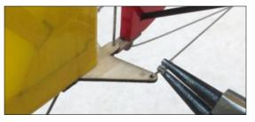
Adjust control wire at <u>left</u> horn. Snug wire until rubber band is just under tension.
