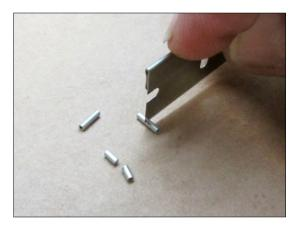
Cut a 30 in. length of supplied stainless rigging wire. Slide one crimp onto wire.
