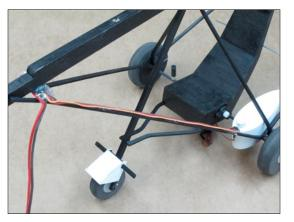
**Rudder Rigging:** Trim a control horn as shown for the rudder servo.
