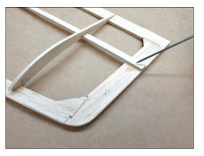
Fit Leading Edge W4 and bond to W1 and ribs. "Arrow" on leading edge indicates position at wing center.
