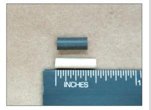
Slide tube onto dowel and secure with thin CA.
