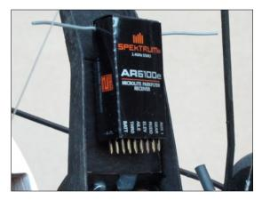
Remove connector from radio lead and female connector from a 3" extension [EFLREX3L]. Trim wires to total length of 8 in. and solder.
