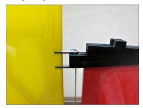
Open mount holes in bottom of horizontal stabilizer with a hobby knife or razor blade.
