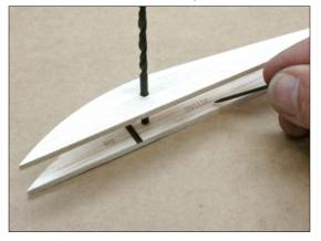
Laminate ribs R1 on each side of the R0 assembly, again using 1/8 in. drill bits to align.
