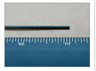
Using 1/32 in. wire, make a 90 degree bend 1/8 from one end. Trim fitting to 1 in. Make two pushrod fittings.
