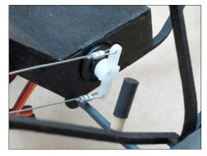
Route control wires above tail rigging and through rudder horn. Upper cable goes to the left horn, lower to the right. Center rudder, draw wire snug and crimp and trim excess. Secure all crimps with a drop of medium CA.
