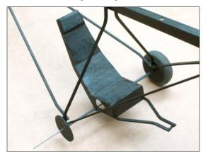
Finally, slide remaining wheel onto axle and make another 90 degree bend 1/8 in. from end. *Ensure bends at each end of the axle are in the same direction.*
