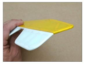
Open slot for the elevator control horn on the lower side of the right elevator. Fit control horn E6, ensuring that it is perpendicular to elevator. Secure with thin and medium CA.
