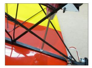
Bend tail skid per plan, fit to hole in rudder horn, and bond with medium CA.
