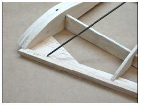
Cut 1/8 in. carbon strip to length and bond to trailing edge with medium CA.
