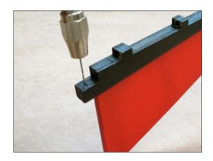
Fit ply rigging tab F10 in slot in ply hinge F9.
