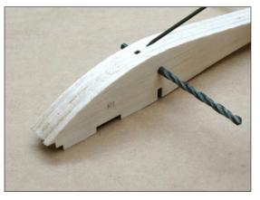
Start with left wing. Fit spar S1 to center rib assembly. Ensure that spar seats snug against R1. Tack glue with thin CA.
