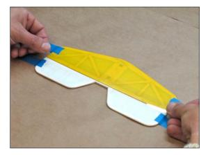
Ensure there is adequate "down" travel. If not, remove tape, increase gap between surfaces slightly, and re-tape.
