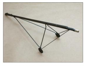
Using a length of 0.045 in. wire, make a 90 degree bend 1/8 in. from one end. Cut wire to length indicated on landing gear plan.
