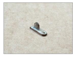
Tack glue rudder hinge assembly to base of vertical stabilizer.
