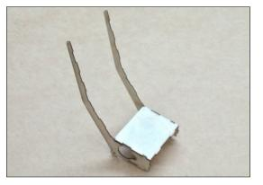
☐ ★ Fit seat front S2a (S2b if building for AR6400) to assembly. Tack glue.
