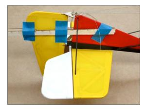
Center servo electronically. Adjust control wire at <u>right</u> horn, removing slack, and crimp to final length.
