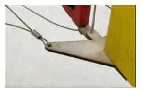
Attach control wire to supplied connector [SIGSH445], snug up and crimp.
