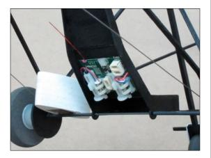
☐ Make an extension for the speed control by soldering 6 in. wire leads to a 3-pin connector available from StevensAero. Configure color coded wires as shown.
