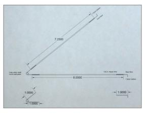
Insert 'V' shaped fitting into one long and one short carbon tube. DO NOT GLUE. Tape assembly to drawing on plan.
