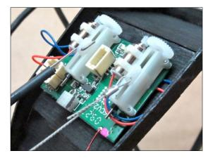
Route control wire above tail rigging and through <u>right</u> side of rudder horn. Center rudder and snug wire. Do not crimp yet.
