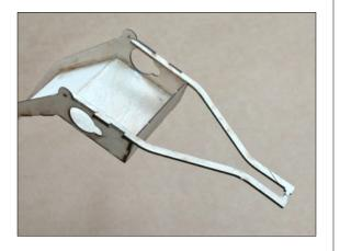
Seal seat assembly with two light coats of Deft and paint desired color.
