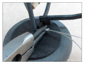
Pass wire through hole in rigging tab at base of vertical stabilizer. **Do not bond to tab.**
