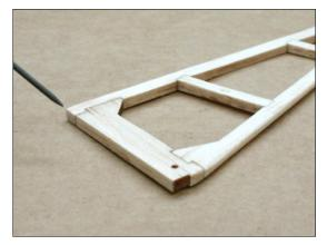
Cover vertical stabilizer. Remove covering from top edge of stabilizer to allow wood to wood bond with fuselage.
