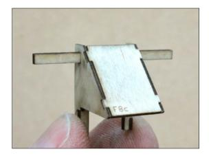
Seal strut/nose wheel assembly with two coats of Deft and paint desired color.
