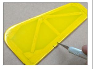
Fit ply hinge pieces R5 in slots. **Do not glue at this time.**
