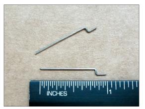
Install metal pushrod ends <u>first</u> to control horn and servo. Use outer most hole at control horn.
