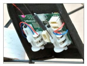
Center elevator both electronically and mechanically. Then retain position with a drop of medium CA glue where push-rod, metal, connector, and heat-shrink tube meet.
