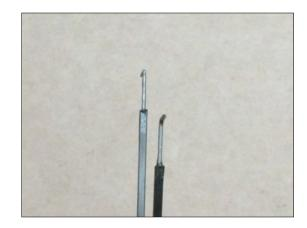
Test by pulling on the fittings with moderate pressure. If any fitting pulls free, coat shaft of wire with medium CA and insert back to original depth.
