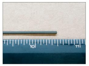
Using .025 in. wire, make a Z bend at one end - refer to plan for size of bend. Trim wire to 1 in. to form pushrod end. Make two.
