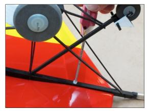
☐ Temporarily attach one strut to axle with Du-Bro RC **Micro II E/Z Link** [DUB920]. Ensure front/rear strut orientation is correct - short strut goes in front.
