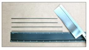
Assemble struts over drawing on plans. Note: Finished strut length is critical to proper wing angle. Check and doublecheck assembly before final gluing.
