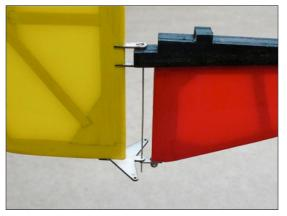
Align hinge pin with center line of vertical stabilizer. Bond hinge tab at vertical fin with medium CA.
