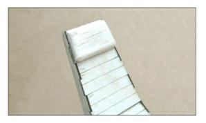
Check alignment of seat. Gently twist assembly or re-fit pieces as necessary. Bond all joints with medium CA.
