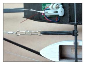
Fix rudder in center position by trapping between two sticks taped together.
