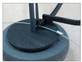
Pass wire back around strut. Slide crimp down trapping end of wire.
