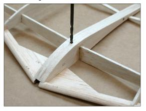
☐ Install 4-40 blind nut through hole from the top of the rib. Nut may be recessed slightly to facilitate smooth covering. Secure blind nut with thin CA around edges of flange.
