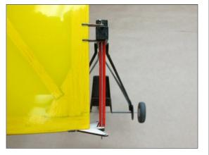
☐ Hinge pin may be left to float free, or may be secure by CAREFULLY placing a drop of medium CA at top. *Ensure CA does not bind in hinge fittings!*
