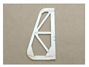
Follow instruction on plan set to lightly sand rudder in preparation for covering. *Do not round off rudder horn mount area.*
