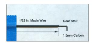
Remove strut assembly from plan and check alignment of fittings. When satisfied, permanently bond wire to carbon with medium CA.
