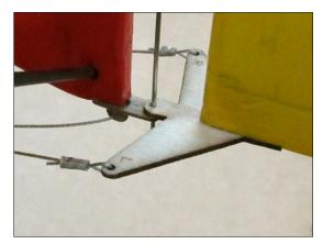
Elevator Pushrod: Trim a control horn as shown for the elevator servo.
