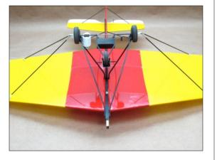
☐ **Tail Rigging:** Optional - Cut 1/16 dia. x 1/4 in. aluminum tube in half to form rigging crimps. Plenty have been provided should you wish not to reduce this part's size.
