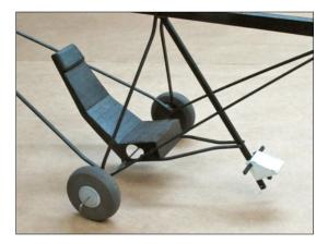
Nose Wheel: Using a length of 0.045 wire, make a 90 degree bend 1/8 in. from one end. Trim wire to 3/4 in. length to form front axle.
