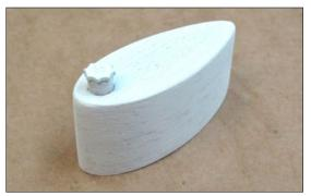
Mount tank on left axle as shown. Tank is tipped forward slightly on full size aircraft. Bond tank to axle and strut assembly with medium CA.
