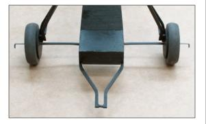
Center axle in seat assembly. Bond axle to hubs with medium CA. *Ensure bends at axle ends point down as indicated on landing gear plan.* Do not bond seat to axle at this time.
