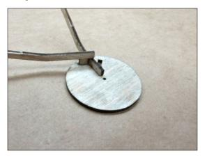
Fit forward strut F2 to hub, trapping F3. Tack glue with thin CA.
