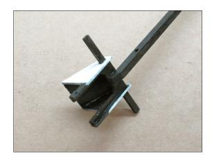
Fit left and right strut assemblies to slots in main fuselage boom as shown. Tack with medium CA glue.
