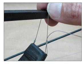
With seat rigging installed we find it helpful to file a small notch where rigging crosses top of fuselage boom to prevent the rigging wire from causing binding when fitting the wing to the fuselage.
