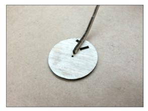
Fit rear strut F4 to hub, trapping F3. Tack glue with thin CA.
