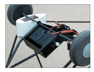
Mount Spektrum AR6100e or AR6110e receiver behind seat with small amount of hot glue or double sided tape.
