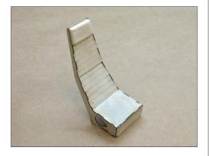
Fit seat struts F7 to side and front as shown. Ensure struts are in the same plane as the base of the seat. Bond with medium CA.
