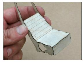
Fit upper back rest S5 between sides, ensuring etching faces forward, and tack in place.
