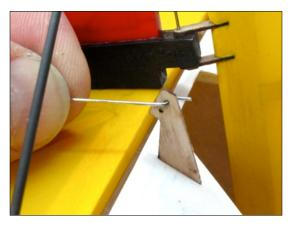
☐ Join fittings to pushrod with a 1/2 in. length of heat-shrink tube. Shrink tube using a fine tip soldering iron.
