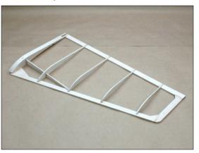
Fit rear spar S2 to ribs. Square wing on table and bond. NOTE - tip of spar rests ON TOP of wing tip.
