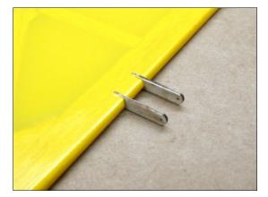
Remove covering from control horn mount at base of rudder.
