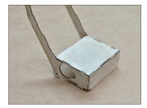
Gently pinch sides together and fit lower back rest S4. *Ensure etching faces forward.* Tack with thin CA.
