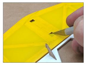
Fit horizontal stabilizer to tabs on F1. *Ensure that stabilizer is horizontal and perpendicular to rudder.* Bond with medium CA.
