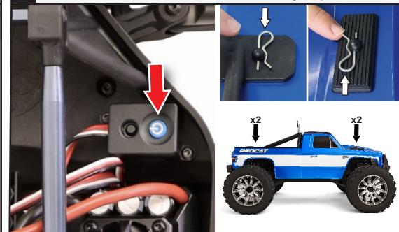
**NOTE:** You can also operate the ON/OFF button by reaching under the body behind the front right tire.
