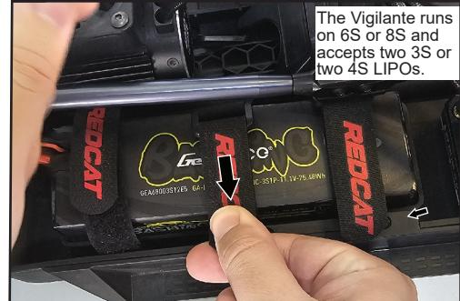
**4.** Plug in both batteries. CAUTION! Do not turn on the ESC yet!
