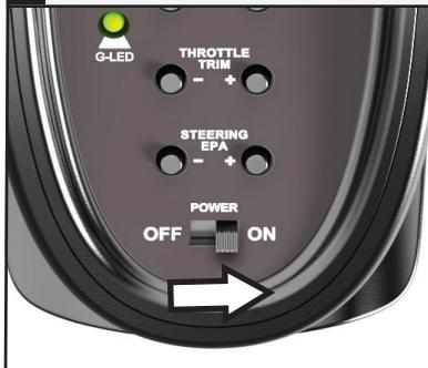
**6.** Power on the ESC and secure the body in place.
