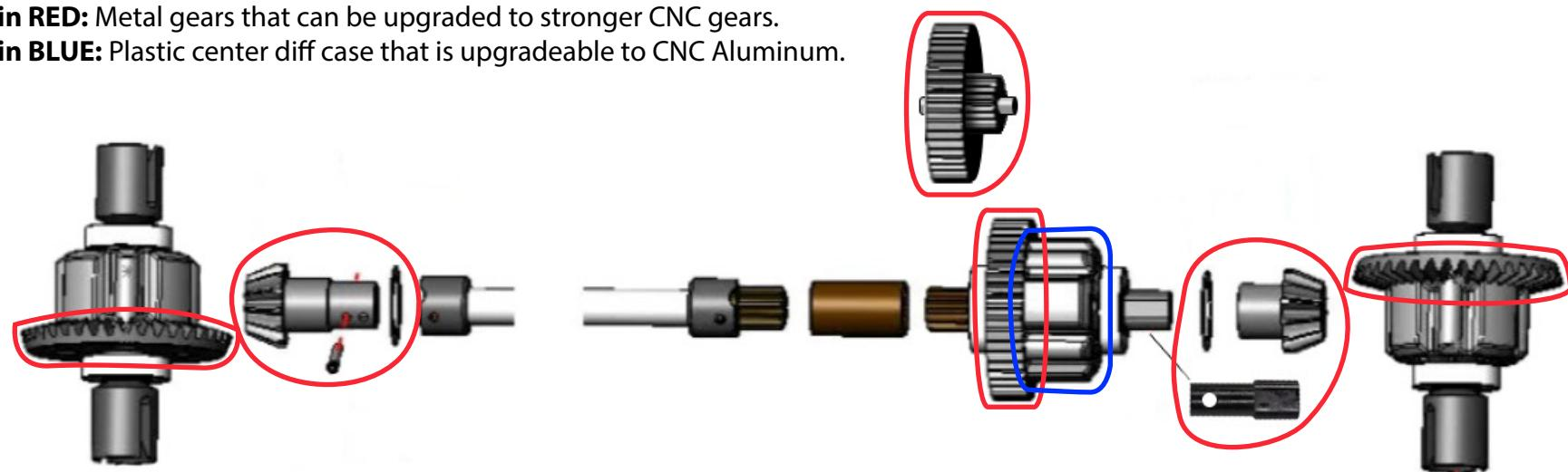
If your Vigilante has a **CNC Aluminum Center Differential Case (RER39156)**; it already has the CNC gears installed and is the latest version of the vehicle. The earlier versions of the Vigilante have a plastic center differential case (shown in the diagram above) and powdered metal gears.
