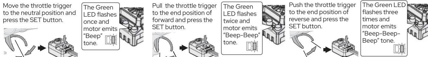
3. To set the neutral point, leave the throttle trigger at the neutral position, press the SET button. The RED LED dies out and the GREEN LED flashes 1 time and the motor beeps 1 time to accept the neutral position.
