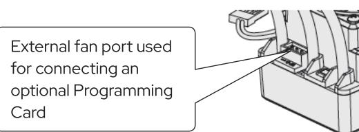
**Attention!** The programming port of this ESC is also the fan port, so you need to unplug the fan first and then plug (one end of) the programming cable into the PRG/FAN port. The other end of the programming cable plugs into the ESC port located on the LED program box. Do not use the throttle control cable, that plugs into the receiver, on the ESC to connect the program card, otherwise the program card will not function.
