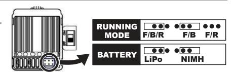
Inserting the jumper into the two right pins on F/B to achieve the "Forward/Brake" (F/B) running mode. It is recognized as a racing mode. In this mode, the vehicle will only go forward and brake.
