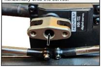
**10.** Adjust channel 3 endpoints so that when channel 3 is pressed, the servo horns go from horizontal to vertical. (see Page 6 of this manual "End Point Adjustments" and "Mode Switching") Attach the main center rods to the double sided servo horns.
