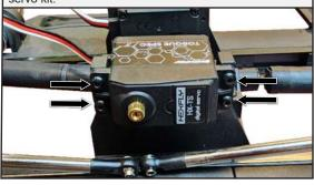
**8.** Using the Y-adapter included in the dual servo kit, connect both servos and put them into your preferred channel on the receiver. When using the included Redcat RTX-4C radio, put the Y-adapter into channel 3.
