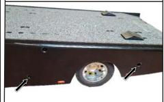
**4.** Remove the 2 screws that hold the exhaust clamps on. One screw per clamp. Remove the on/off switch and then pull the bed assembly straight up and set it to the side
