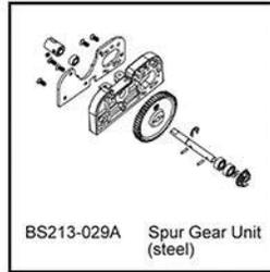
BS213-029A Spur Gear Unit (steel)
