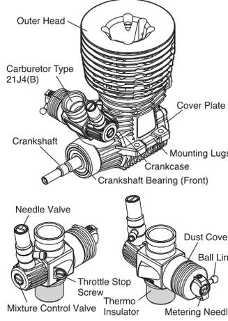
**■ CARBURETOR CONTROLS - STANDARD POSITIONS (POSITIONS WHEN THE ENGINE LEAVES THE FACTORY)**
