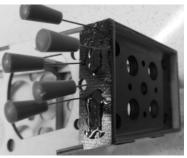
Apply some epoxy over the firewall tabs and along the rear seam of the plates, especially if there is some gap between the plates and ply.
