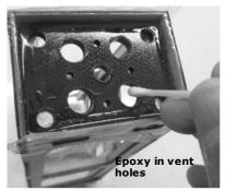
7. Using a cotton bud apply a thin layer of epoxy in the firewall vent holes except the mounting holes. wipe off any excess where the motor is mounted
