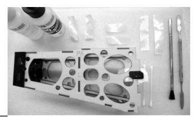
**1.** Prior to installation **go over all pre-glued joints** with white carpenters' glue or epoxy **(except firewall!)** to ensure they are properly bonded and no gap between the parts is present so it will be able to withstand the torque created by the powerful Thrust 50 motor.
