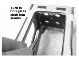
**6.** Cut two fiberglass straps approximately 70 mm long. Brush epoxy over the outside top and bottom sides including corners. Then place each strap over and brush a thin layer of epoxy on top as you did before. Continue by brushing a bit of epoxy over the front frame and sides of plates.
