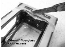
9. Please, make sure to follow the KMX instruction manual to complete the motorbox installation to the fuselage. use only epoxy and make sure you cover the **entire** CF rods, especially the one at the front. Spot gluing will **NOT** work and will allow excessive flex of the front bulkhead which can cause the motorbox to fail under loads.
