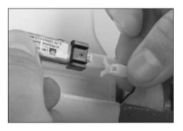
**Note:** Always disconnect the Li-Po from the receiver of the airplane when not flying. Failure to do so will render the battery unusable.
