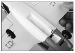
**Note:** You can adjust the nose gear height by slightly pulling out the nose gear strut to create a more positive angle of attack, and more prop clearance.
