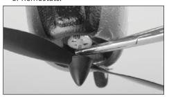
2. Remove the propeller by turning it counterclockwise on the threaded shaft
