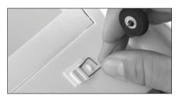
Gently slide left and right mainlanding gear into plastic mounting clips on the bottom of the wings, orienting the struts toward the front of the airplane as shown.
