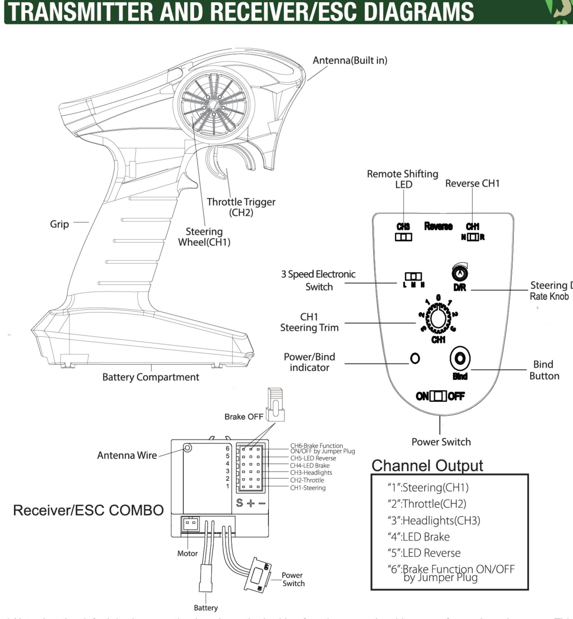
\* Note that the default brake operation is to have the braking function operational between forwards and reverse. This means as you release the throttle trigger to neutral there will be some braking action occurring. If you do not want this braking action please install the jumper plug as shown.
