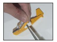
Place the exposed section on the surface making sure that your decal is properly aligned on the part. Peel and cut backing off in stages.
