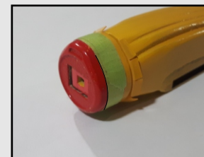
Tape off first 1/8" of cowl and paint red
