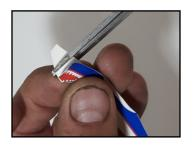
For the large decals, remove about a 1/4" of the backing and cut off with scisors.
