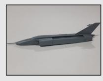
Once shaping is complete put a primmer on all surfaces to seal the wood. You will want to apply around three coats. Sand with 320 grit sandpaper between coats. Once good coverage has been obtained, paint all surfaces white.
