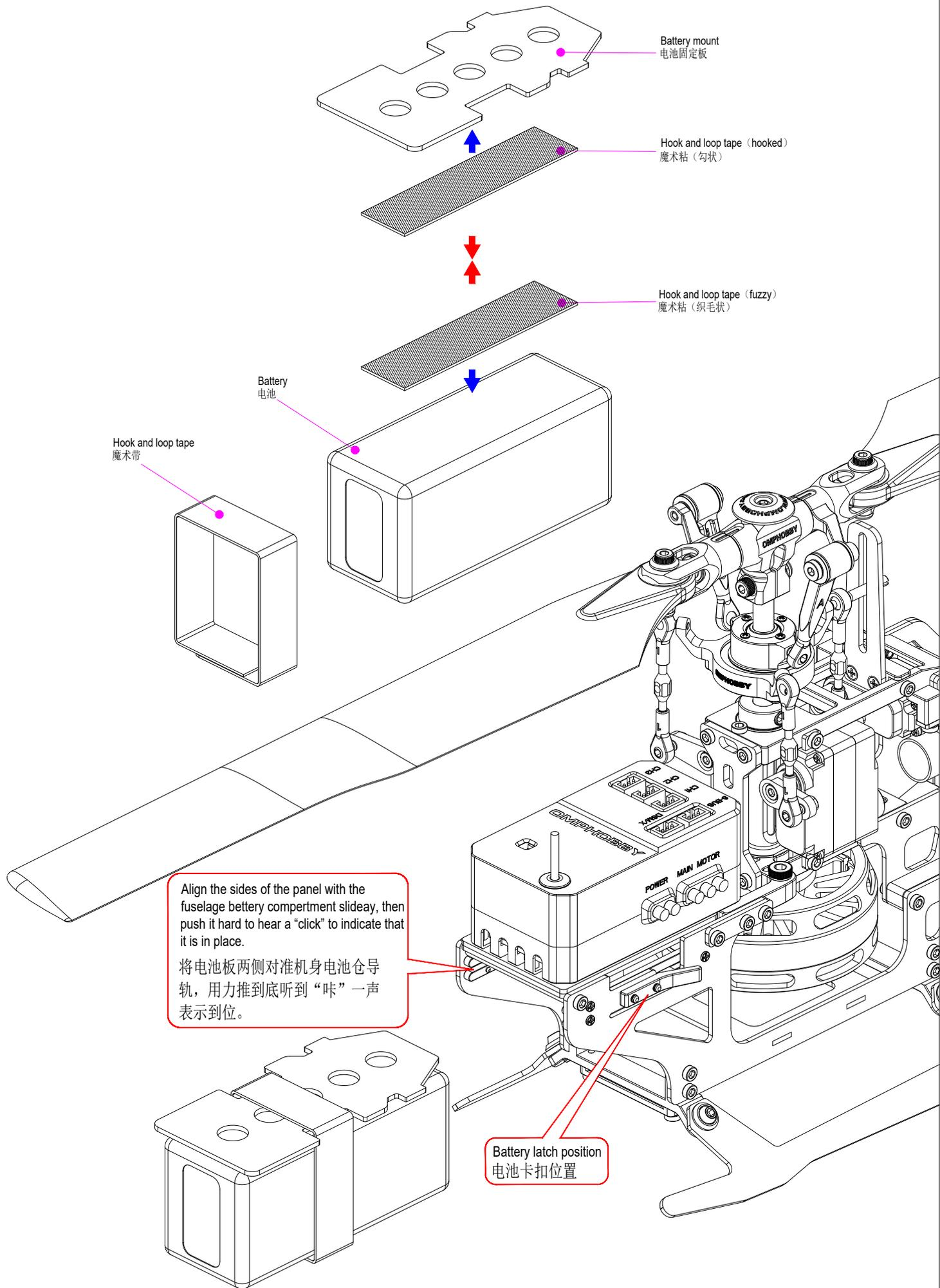
Align the sides of the panel with the fuselage battery compartment slidey, then push it hard to hear a “click” to indicate that it is in place.
