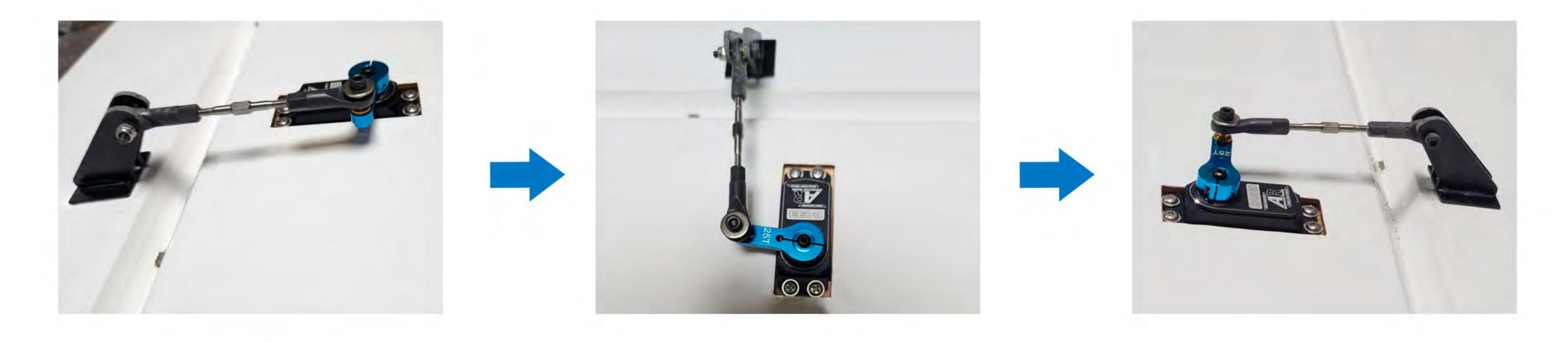
② Gluing in the elevator horns
