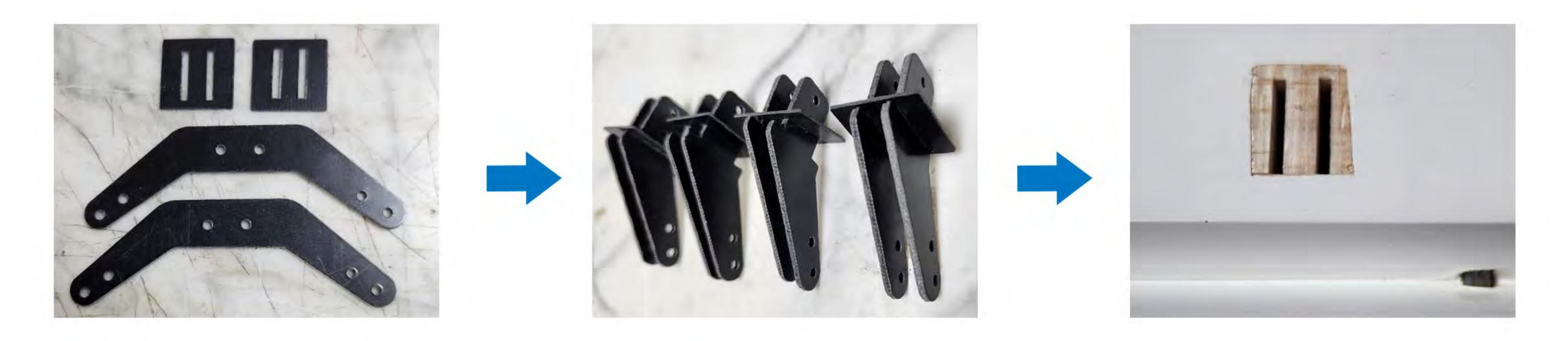
② Use sand paper to scuff up the bottom of the horns for a good glue bond. Try to insert it into the mounting slots to adjust the position first.
