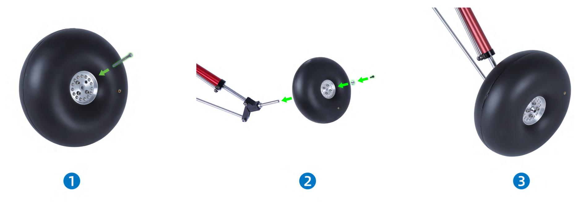
Install the tail gear with the provided socket head screws and washers, using threadlocker.
