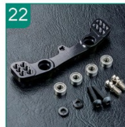
210590R/BK RMX 2.0 Alum. steering joint plate (black)
