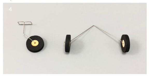
Thread the wheels into the landing gear steel wire, and bend the outer end of the steel wire with pointed nose pliers. Or: put 2mm heat shrinkable pipe into the outer end of steel wire, and fix the pipe with glue to hold the wheels.
