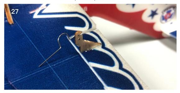
Attach the pushrod clip on the same hole of aileron servo arm.
