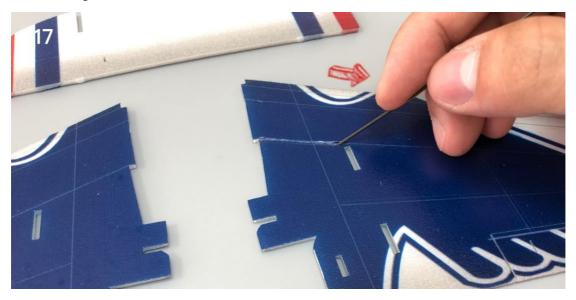
The wing can be bent down along the center longitudinal scribe.
