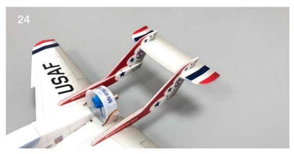
Paste the sticker on the top of the fuselage to form a hinge connection for the hatch cover to be turned over. Glue can be used at the hinge joint to increase strength.
