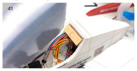
Battery and receiver are fixed in the cabin with Velcro.
