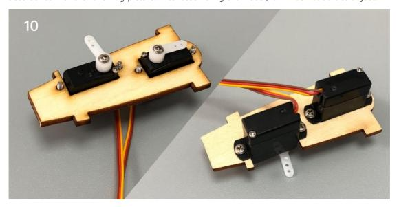
Combination of side plate and servo base.
