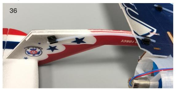
Attach the wire clip to the control horn, and connect it with the steel wire with heat shrinkable
