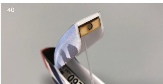
Install magnet base on the fuselage.
