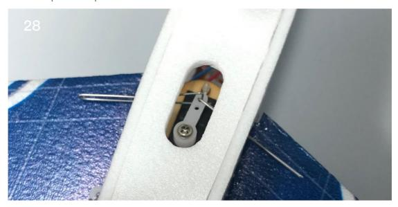
Fix the aileron duct seat with glue. The distance between the two seats and the fuselage and aileron control horn are 30mm.
