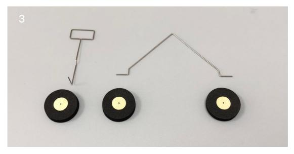
As shown in the figure, bend the center part of the front landing gear backward to realize the shock absorption function.
