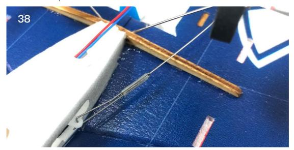
Fix the magnets on the magnet bases with glue.
