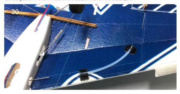
Thread the steel wire into the duct and check for smooth movement.
