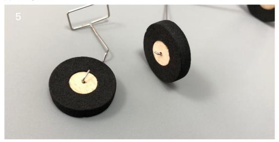
Bend the top fixed seat of nose landing gear 90 degrees to the right.
