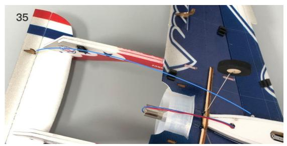
Use 502 glue to fix an 80mm duct on the base.
