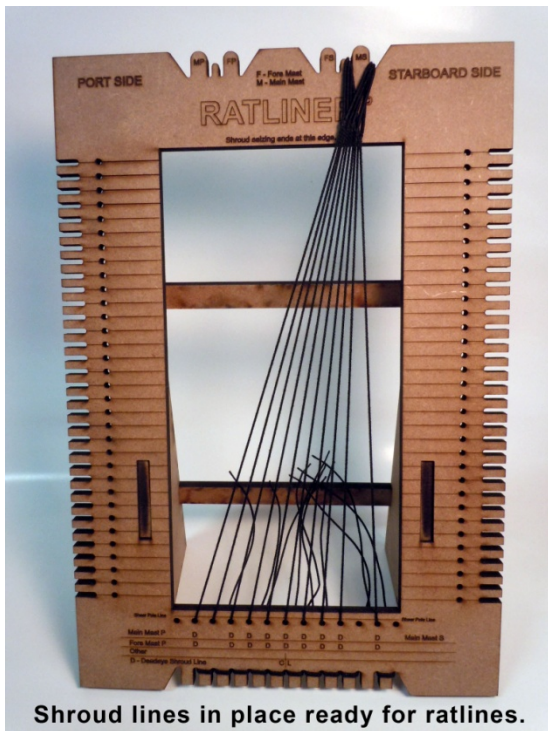
G. Shroud lines in place ready for ratlines.
