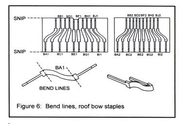
The staples pass through the rails and are bent over on the inside to secure them. Their locating holes have been laser cut but will need to be drilled through the box sides. Use a #72 drill and drill all 40 holes.
