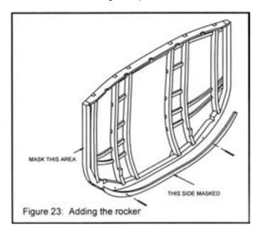
Mask the area on the ends of the coach sides which will later receive the coach end panels. Refer to figure 23. Mask the hinge mortises on the coach sides and the doors. The sides and doors may now be finish painted inside and out.
