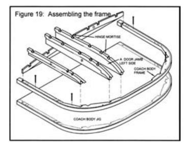
Now fair the structure to conform to the design curvature of the side. Use a sanding block and a strip of 1/16" x 1/8" called a batten to check the progress. Fairing is the process of shaping the edges of the parts and the notches so that they conform to a smooth curve allowing the paneling and rails to lay on the structure with intimate contact. Carefully sand the stiles and frequently check with the batten until you are satisfied with the fairness. Refer to figure 20.
