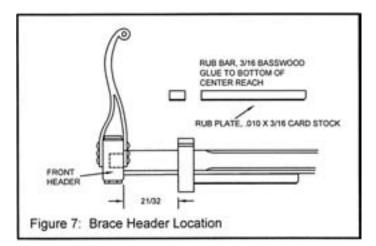
Locate the rub bar on board SC-1. Cut a piece of card stock 3/16" wide and 1 1/16" long and glue to the bottom of the rub bar. This is to simulate an iron plate. The rub bar may be finish painted before gluing to the center reach. If you have pre-finished the reaches scrape off enough paint for a good glue bond.
