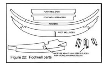
Mask the outboard side of the rockers by laying the part on masking tape and cutting around it leaving only the face of the rocker masked. Cut 4 pins about 3/8" long from 1/32" dia. brass rod. Use these to locate the rocker temporarily on the well side. Do not glue. We are using the rockers to mask the gluing surface while finishing the foot well assembly. Also cut thin strips of masking tape and mask the ends where the end panels of the coach will seat later.
