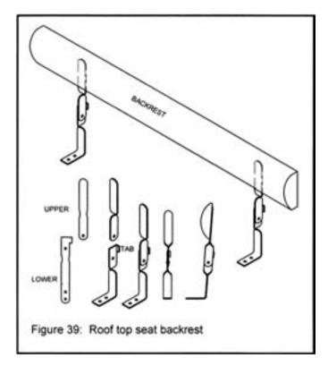
Refer to figure 39. If you have not finished the seat and back cushions in a previous step, do so now. These pieces are on board SC-1. Locate the brass backrest brackets, upper and lower. Note that there are small notches on the lower bracket indicating where the bend is to be for the foot. Use pliers to make the bend. Both the upper and lower brackets have a scalloped indentation locating the position of the 90 degree twist.
