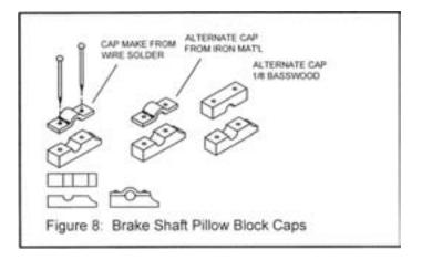
Another method is to use the iron material caps on board SC-11. Also the cap blocks on board SC-4 may be used. Drill and pin the caps of your choice. Check that the brake shaft rotates freely. Adjust as necessary.
