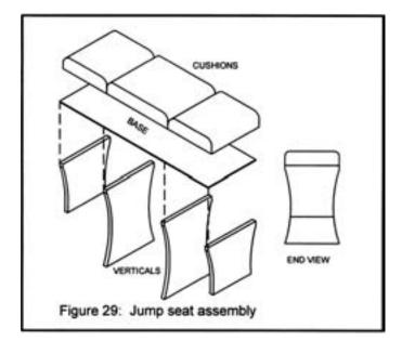
On full size coaches the outboard sections of the jump seat were hinged so that they could be swung up and over the middle seat to facilitate ingress and egress of the passengers.
