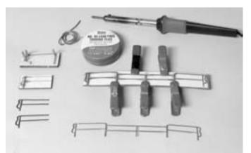
Photo 26: Forming and soldering jigs
