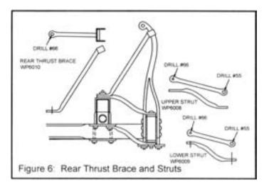
In like manner drill and fit the lower strut from the rear bolt on the inboard axle clip to the bolt coming down through the rear header. Square nuts can now be glued to the lower strut keeping it in place.
