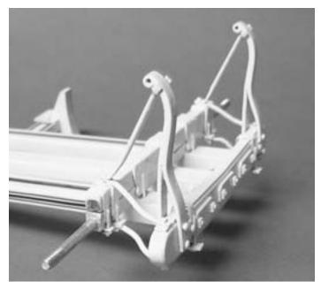
Photo 3: Rear struts and thrust braces
