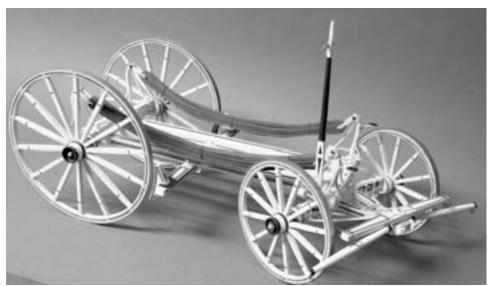
Photo 13: Assembled undercarriage and running gear
