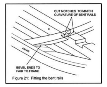
In a similar manner install the lower bent rails. Also found on board SC-7 are the door sills. Install a door sill and we have completed the framework for the left side. Use a sanding block to fair the structure in preparation for the paneling.
