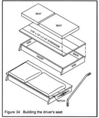
Cut notches for the driver's seat braces as shown in figure 34. This assembly may now be masked and finished. Mask the rear of the assembly where it will be glued to the coach body. Mask the inner sides of the
