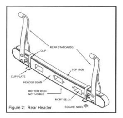
Glue on the top and bottom iron plates and drill the vertical holes as shown with a #55 drill. Drill all holes and Install the rear header standards (WP6003 and SP6004) just as you did for the front header. Then prepare and install the clips, clip plates, and square nuts.
