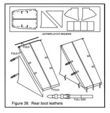
The front boot leather glues to the inside of the driver's seat ends. Refer to the illustration on plan sheet 4. The leathers for the prototype model were given and wash coat of thinned burnt umber acrylic for a more realistic leather look.
