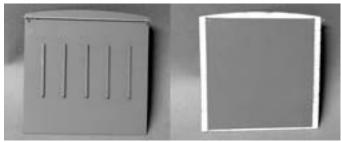
Photo 24: Coach body rear end panel, masked and finished front and back.
