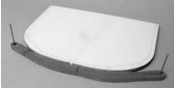
Photo 10: Method of shaping the thorough braces.
