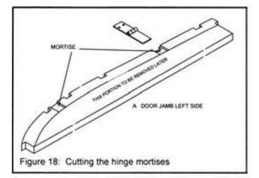
The door jamb parts have a laser engraved line defining the mortises. Cut the mortises about 1/32" deep. Test fit a hinge and adjust the depth so that the hinge is flush with the surface of the jamb. Later we can adjust the mortise depth when the doors are fitted if necessary. For now we want to accomplish the majority of cutting the mortises while the jamb is easily accessible.
