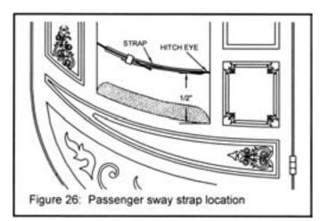
Refer to figure 26 and drill #66 holes ½" above the window bottom. Use a pin vice and drill the holes at an angle so that your vice does not mar your finish. This will also give the hitch eyes some resistance from pulling out. Insert the hitch eyes and bend to align with window.
