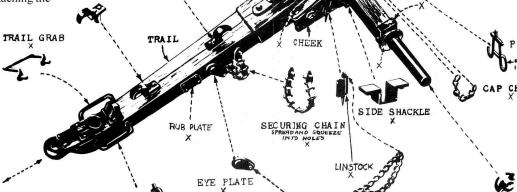
(2) Apply cement to SHIMS (discs) on inside of CHEEKS and in holes in TRAIL. Push CHEEKS into TRAIL holes. Make sure that CHEEKS are in line, level and square.
