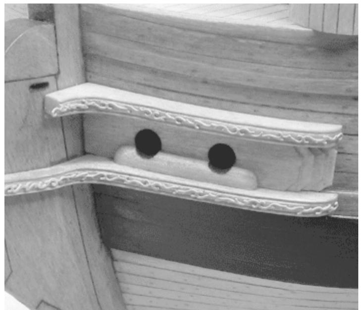
Drill the hawse holes through the hull. Be careful not to mar the laser cut holes in the second layer. Drill smaller holes and then carefully enlarge them with a round needle file. The bolster is then added as the last layer. This is the small piece that sits under the hawse holes.
