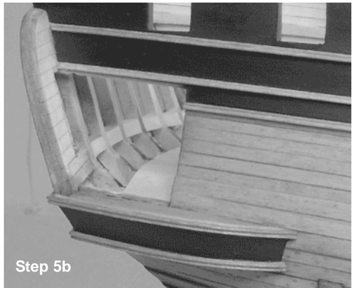
give the finished model its delicate and elegant look that was so common with contemporary models of the time. Once the inboard side of the hull is planked, it will be between 3/16" and 7/32" thick. On the real ship, this would translate to 1 foot – 14" thick along the cap rail. When you finish fairing the hull inboard, you can move ahead to step six below in order to complete the stern and quarter galleries.
