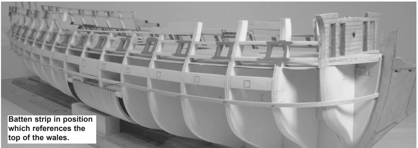
**Batten strip in position which references the top of the wales.**
