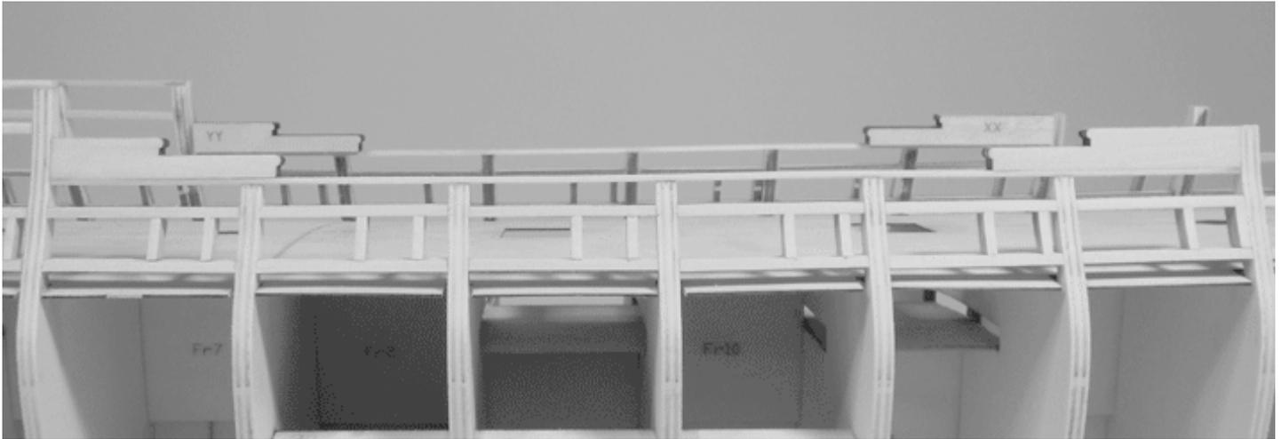
**Measuring the sweep port strips to fit into position after establishing a clean run for them with a batten.**
