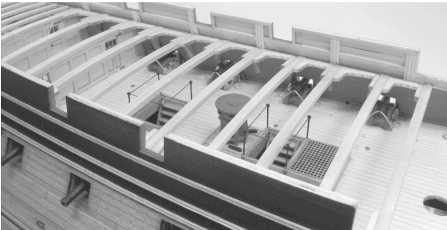
al stanchions of varying lengths are used throughout the kit. Compare them against the plans. The two stanchions at the back of the companionway are glued on the diagonal to make positioning the railing easier. All four should be glued into the top of the coamings. Be careful drilling the holes. The coamings are quite thin. Only a small hole is needed.
