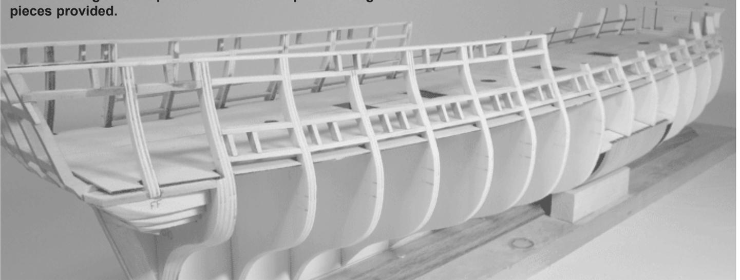
Bridle port bulkhead extension cut free before adding the two uprights to complete the sides of the port.
