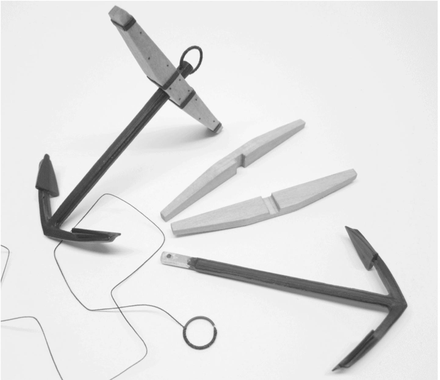
also be simulated on both sides of the stock between each iron band. See the plans for their locations. The bolts can be made with 28 gauge black wire as you have done earlier in the project.
