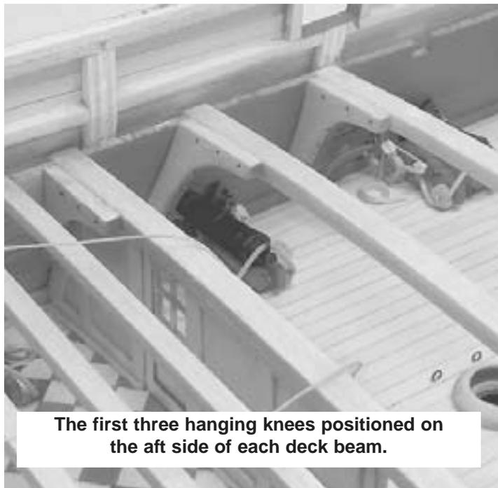
The first three hanging knees positioned on the aft side of each deck beam.
