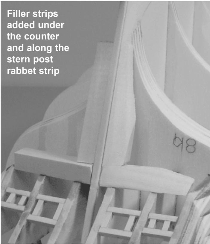
x 3/32" strips for the uprights. The sides of the ports should be perfectly vertical. They are not angled. So avoid using the stern frames as a guide since these are on an angle. Once the port uprights are in position you can fair the counter for the last time. This also includes fairing the quarter filler pieces. (DD, EE and FF) They should also be faired so the gentle convex curve is evenly established across the entire lower counter.
