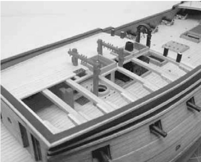
planked on the port side. The cat-beam is the first deck beam that sits against the beakhead. You need to cut small lengths of planking to cover this beam. This will make the surface on the port side level with the starboard side so the catheads (cat tail) can be installed properly.
