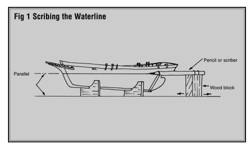
*Scribing the waterline*: This can be done in a variety of ways. One method is to mount the hull so the waterline is parallel to the bench top, then mark the waterline using a height gauge and sharp pencil or scriber (Figure 1). With or without the aid of masking tape, paint the bottom and topside colors precisely to this line. The scribed line acts somewhat as a barrier against transgressions by either color, but a steady hand is needed.
