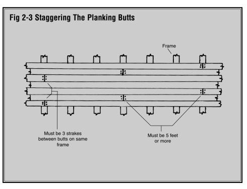
To emulate shipwright practice, stagger hull and deck planking butts. Two or more planks per strake may be necessary to do this. Figure 2-3's pattern is similar to a real ship.
