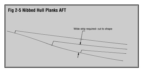
The tapered strake above the garboard must fit over its nibbed end. After cutting the aft end to accommodate the nibbing, spile the remaining portion of the strake. Repeat this procedure for every plank up to the belt line. Remove the batten when it interferes with progress.
