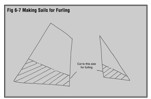
this problem, either proportionally reduce the size of a sail by one-third when using sailcloth (Figure 6-7), or buy a lighter material such as Silkspan (model airplane covering tissue available from Model Expo). Depending on their size, even Silkspan sails may require being reduced by one-third. Test the percentage reduction to determine how much material is needed for a neat, tight furl. Even furled sails need some seams and hems, as these details are visible.
