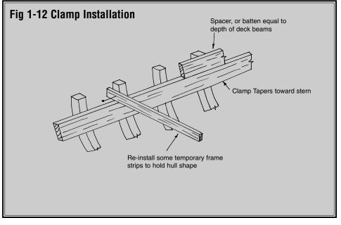
**Note:** Modelers electing not to bevel the inboard side of the frames can glue the clamps directly to their edges. Don't omit the clamps. They are important to the hull's rigidity and support those deck beams not attached to frames.
