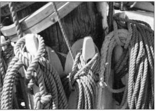
Rigging lines belayed to fore mast cleats.
