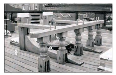
FOREMAST FIFE RAIL undergoes restoration. Note the triple sheaves in the base of each stanchion. Three kevels in the bul-wark are normally used for belaying large lines.
