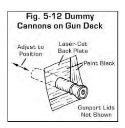
barrels on the gun deck. The hole in the laser-cut box back plate (Stage 1, Step 11) fits the back of the casting. Slide the dummy cannon in or out to position its barrel (Figure 5-12).
