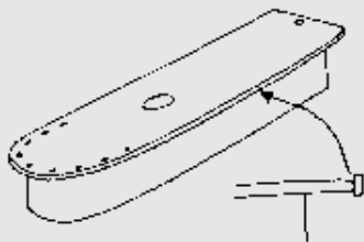
FIG. 12 – Adding the Cabin Top
