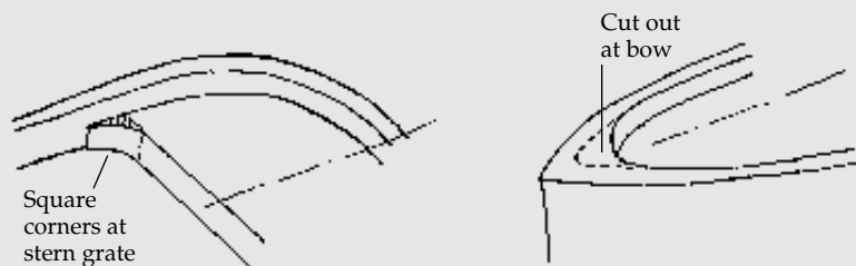
FIG. 4 – Carving the Deck
