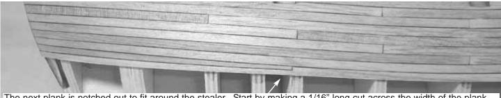
The next plank is notched out to fit around the stealer. Start by making a 1/16" long cut across the width of the plank where it will butt into the end of the stealer. Then gradually taper the aft end to the full 1/8" width as it runs off the stern.
