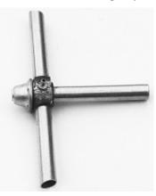
Glue the gear housing assembly to the engine stand. The stand cradle should snug up against the flange on the gear housing.
