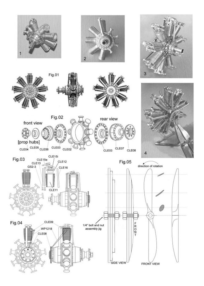
Referring to Fig. 02, attach the front and back crankcase covers (CLE-03) to the crankcase (CLE-02). Note the tiny notches in the castings to help you align the parts. Glue one side in place, then make sure the bolts heads line up on both covers before gluing the second cover in place. Slip this subassembly onto the brass tube (KS-129), which for now, serves as an engine alignment jig. Do not glue the cast parts to the tube.
