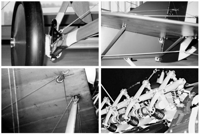
Clockwise from upper left: Landing Gear Shock Cord, Horizontal Stabilizer, OX-5 Engine Cylinder Heads, and Aileron Control Wire Sheave, as they appear on restored Jenny's
